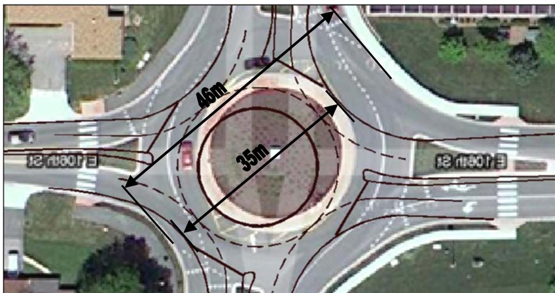
Figure 2: A C-Roundabout alignment atop a typical dual-lane layout from the United States, which is similar to Austroads in terms of space requirements.
