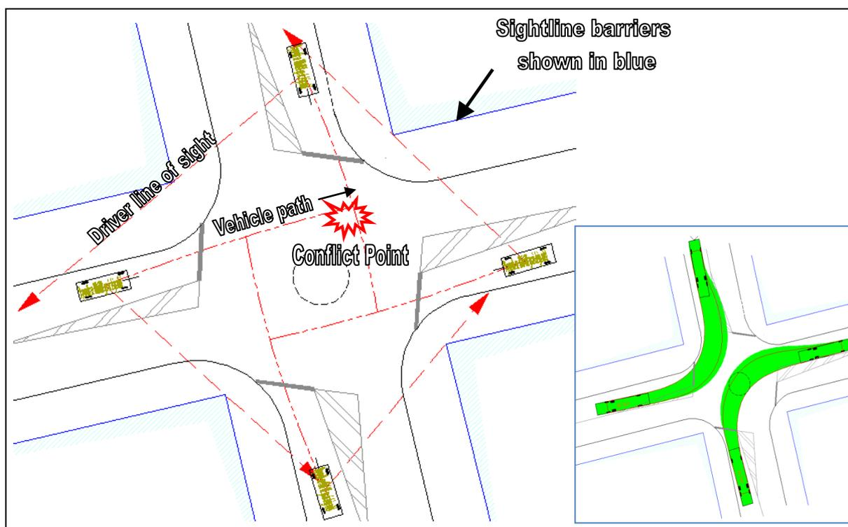
**Figure 4: Concept drawing for a single-lane roundabout (outside diameter approx. 20m or smaller) using sight line restrictions with low mountable or flush central island. Inset is shown large bus tracking.**
